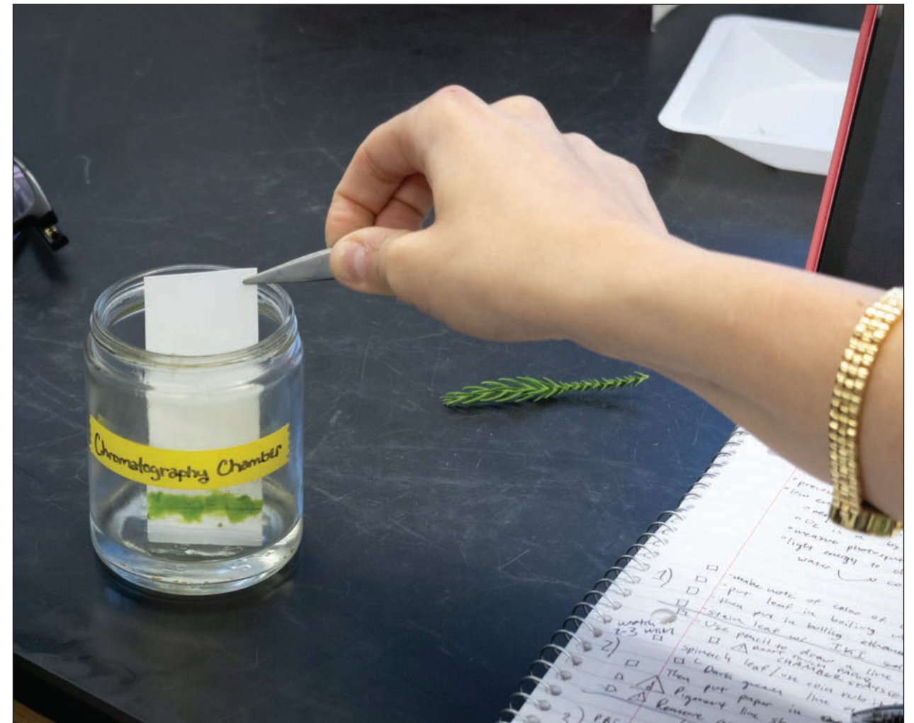
A student dipping their spinach paper into a solvent so the individual pigments separate.
